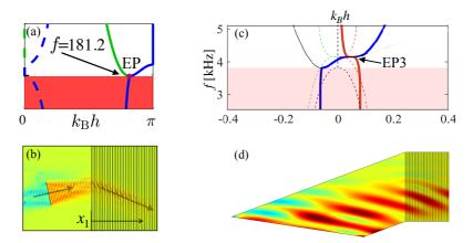
We extend our design and achieve the coalescence of three Bloch modes (EP3) using anisotropic material [Fig. (c)]. We show it gives rise to modes with zero axial group velocity and finite transmittance, known as 'axially frozen modes' [3]) [Fig. (d)]. These modes, previously discovered in 3D dielectric laminates [3], are now accessible in simpler, planar settings in elastodynamics, thanks to the distinct tensorial properties of elastodynamics.
